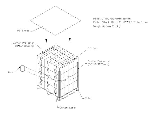
Figure. 8-2 Packing method
