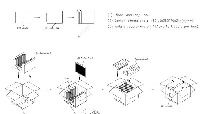
Figure. 8-1 Packing method
