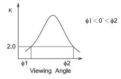
Contrast ratio K vs viewing angle ♦
